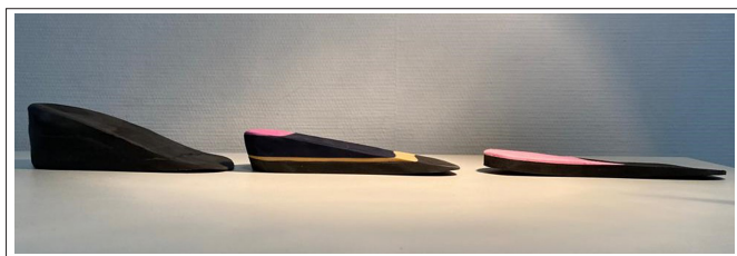
Figure 1. Side view of 1 cm, 2.5 cm, and 5 cm heel wedges made of EVA. EVA, ethyl vinyl acetate.
